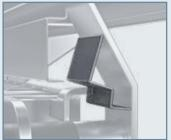
By changing the geometry, the deck retainer is now system-integrated.
